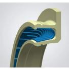
The dual-lip body offers improved sealing performance in virtually unlimited media service and the widest temperature range. Finger spring MSE<sup>®</sup> seals use a cantilever-type stainless steel spring to act as an energizer during low pressure situations. The flanged series dual lip seal is intended for use in rotary applications. The flange helps prevent seal rotation, a major cause in rotary seal failure. Designed for maximum surface speed of 250 ft/min (1.27 m/s) and 4000 psi (276 bar).
