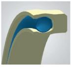
Canted Coil Spring Energized MSE® seals allow for lower seal friction at low pressure. The Canted Coil Spring has a flatter spring rate curve compared to finger and regular coil springs, allowing for more consistent spring force throughout its deflection. The Extended Heel Series is preferred for high-temperature/high-pressure applications. Rod and piston types use one Extended back-up gland width. The Canted Coil spring is intended for temperatures from -270°F to 550°F.
