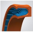
The scraper lip design is best suited for non-lubricated applications where abrasive media are present and where space is limited. The scraper lip keeps abrasive media from getting between the seal and the hardware, thus decreasing abrasion. Available in rod and piston designs.
