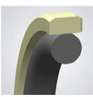
O-ring energized PTFE cap seal offers simplicity and low cost. The Glidetec seal offers bidirectional sealing, low friction and easy installation in compact single-piece glands.
