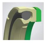
A unidirectional, "self-venting" seal design consisting of a PTFE jacket and an elastomer O-ring energizer. The seal design and energizer allow installation into "closed-groove" configurations for most sizes. The seal can also be complemented with a high modulus backup ring for higher pressures or larger sealing gaps. Along with the "self-venting" capability, the ESE design offers low operating friction along a wide operational temperature range.
