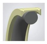
The Advancap<sup>™</sup> rod and piston seals are designed to provide a cost-effective cap seal solution that prevents extrusion and eliminates O-ring spiral failure in dynamic applications. Each seal combines a cap made from Avalon®, our PTFE material, and an elastomeric O-ring energizer.
