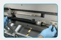
We are FAA-certified to repair Marathon Norco Hold Open Rods. Using OEM-designed tools and equipment, we conduct precise functional tests—including compression and tension load testing—to ensure reliability. As an OEM-authorized MRO station, our team is fully trained to deliver high-quality diagnostics and repairs to the highest industry standards.
